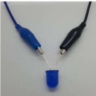
> Connect the shorter leg (the *cathode*) to the GND alligator clip and the longer leg (the *anode*) to the PO alligator clip.
