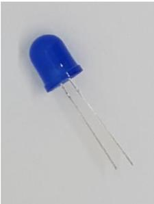
Take a look at one of your LEDs. The legs on it are two different sizes. The longer leg is the positive side (also known as *anode*) and the shorter leg is the negative side (also known as *cathode*).
