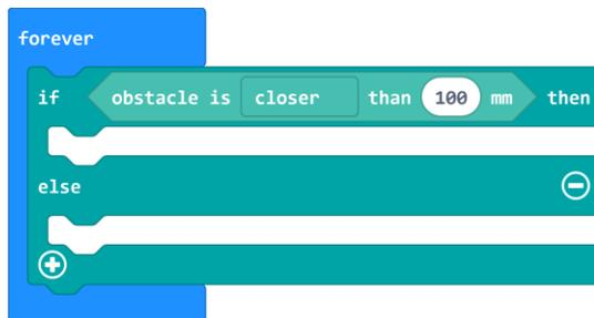
Next, we need to determine what values we want the GiggleBot to be looking for. Since we are using the distance sensor, think about how close you want the robot to get to an object before reacting.
