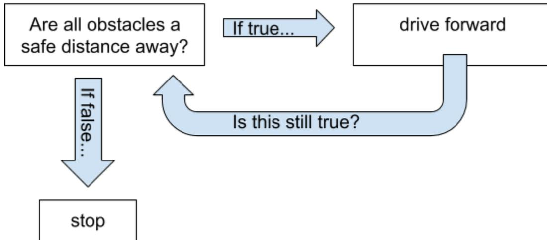
**CAUTION:** If the body of the **while** loop takes a long time to execute (for example, cycling a rainbow for many seconds) then the condition gets tested only after it finished executing. It does NOT get tested continuously. The robot can miss obstacles that way.
