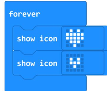
This code will display a beating heart on the micro:bit screen. It will start as soon as the micro:bit is turned on, and will beat until the micro:bit has no power. Transfer this code to your GiggleBot to see it in action.
