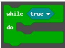
Place a block **while true do** (found under **Loops**) inside of the **on Button A pressed** block .
