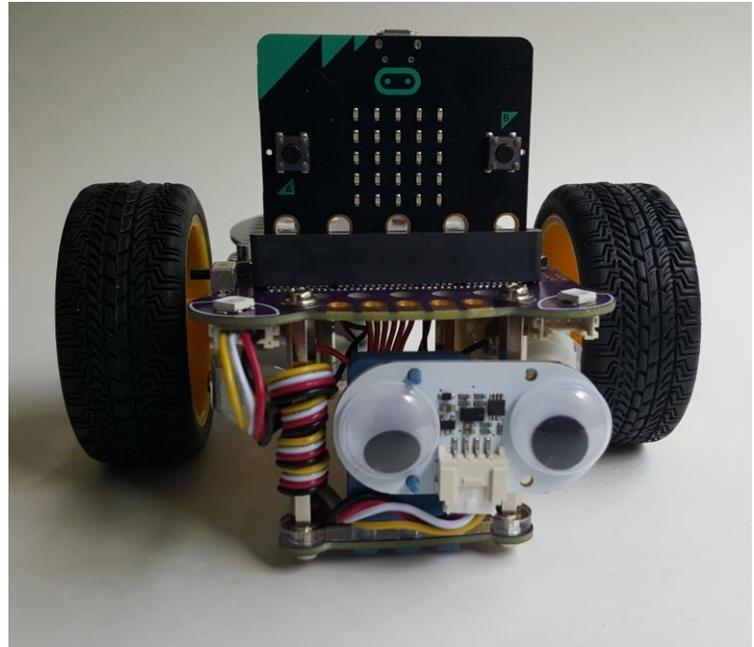
The distance sensor works by sending out a pulse of light in front of it. It then measures the time it takes for the light to reflect off of something and return to the sensor to measure how far it is from an object. Using this sensor your GiggleBot can detect obstacles and react to them.
