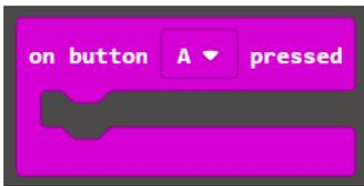
Let's begin by moving an block **on Button A pressed** (found under **Input**) to the workspace. We used this block in Mission 2: Light Show to initiate all or part of a program to control the lights on the GiggleBot. This time we will use it to start a different type of program.
