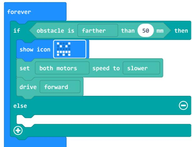
Next, we will choose what the GiggleBot will do when an object is detected less than 50 mm away. Instead of having the GiggleBot fear obstacles, this one will “attack” them gleefully. What blocks could you place after **else** to tell the GiggleBot to “attack” the object? An example is shown here.
