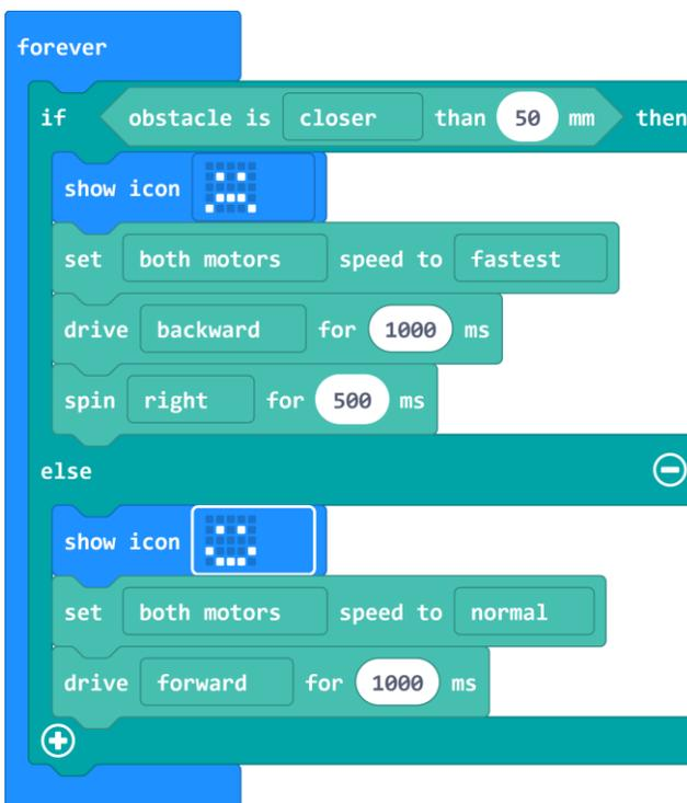
> Inside the **if then...** block opening, add blocks to tell the GiggleBot what to do if it gets closer than \_\_\_\_ mm to an obstacle. In this example, the GiggleBot will display a sad face, drive backwards quickly, and then turn around when an obstacle is detected that is closer than 50 mm.
