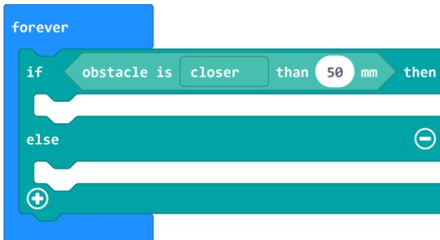
> In this example, the value was changed to 50 mm. This means the GiggleBot will do an action when the distance sensor reads a value less than 50 mm, in other words the GiggleBot will react if an obstacle is within 50 mm of the distance sensor.
