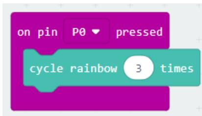
In this example, the GiggleBot will cycle a rainbow three times on the smile LEDs when **P0** is pressed.
