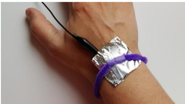
**Pro tip:** Create a wristband for the GND pin so that you only need to touch the P0, P1, and P2 pins. The GND pin will already be connected since it is touching your skin! One way to do this is to put a piece of foil or dough underneath a bracelet made from a pipe cleaner.
