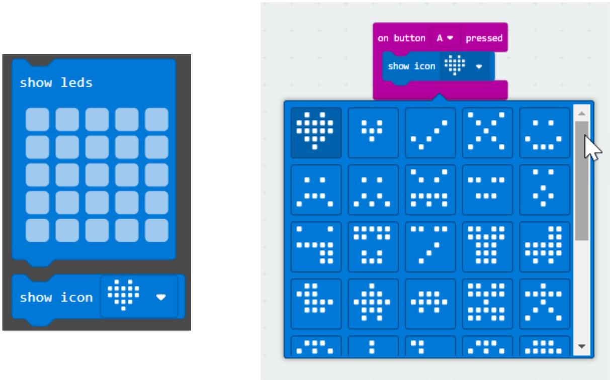
Here is an example of a program where you can change the icon displayed on the micro:bit using the buttons. This example will make the micro:bit smile when button A is pressed, and pucker when button B is pressed.
