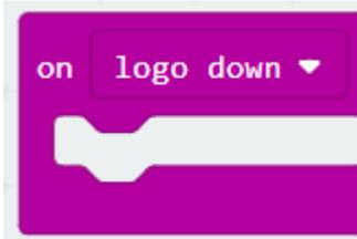
**GiggleBot** -This is when the GiggleBot, with the micro:bit attached, is upside down. The wheels are facing up and the top of the GiggleBot is facing the ground. Usually not a good position.
