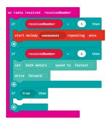
> Add one last **if true then** \_\_ block inside of the on radio received block.
