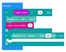
Place this if \_\_ then \_\_ block underneath the first if \_\_ then \_\_ block for the light sensor readings.
