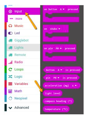
The GiggleBot will display the light value as seen by its own micro:bit. Play with the light level around the GiggleBot: use a blanket to create a shadow, or bring it close to a light source. Verify that the displayed number does change accordingly.
