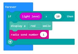
We will send the message by sending a number to the additional micro:bit. Later, we will tell the additional micro:bit what to do when it receives each of the numbers. Connect a radio send number \_\_\_ block below the display red smile block. Change this number to 1. Now your GiggleBot will react to the lights being turned on!
