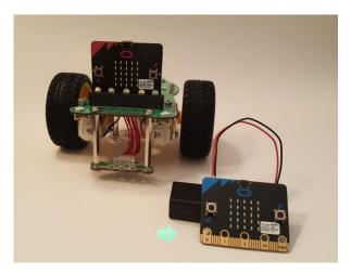
Also be sure to plug in the distance sensor to one of the I2C ports and to connect the speaker using alligator clips.
